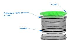
Install the telescopic gasket (shown in the diagram as "Gasket") provided with the hatch into one of the three seal sockets in the telescopic frame of the cover. Then, press the hatch casing into the well extension to the desired depth. To facilitate smoother movement of the hatch within the seal, lubricate the sealing surface of the gasket with a sliding agent beforehand. The telescopic hatch casing can
