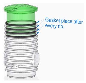
After cutting the well extension to the correct size, reinstall the telescopic gasket onto the upper edge of the extension. Then, press the hatch casing into the gasket according to point 4.1
