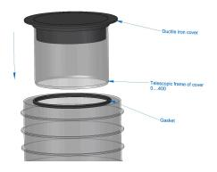
Install the telescopic gasket (shown in the diagram as "Gasket") provided with the hatch into the opening of the well extension, ensuring that the gasket covers the entire upper edge of the well extension. Press the telescopic hatch casing (shown in the diagram as "Telescopic frame of cover") into the gasket installed on the upper edge of the well extension. To facilitate smoother movement of the hatch within the gasket, lubricate the sealing surface of the gasket with a sliding
