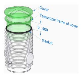
The gasket provided with the hatch (shown in the diagram as "Gasket") should be installed on the upper edge of the well extension so that the gasket covers the entire upper edge of the well extension.
