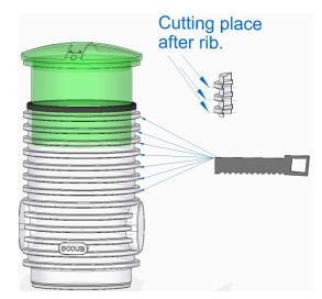
In case the telescopic capability provided by the hatch casing is not sufficient, it is possible to shorten the well extension according to the illustration.
